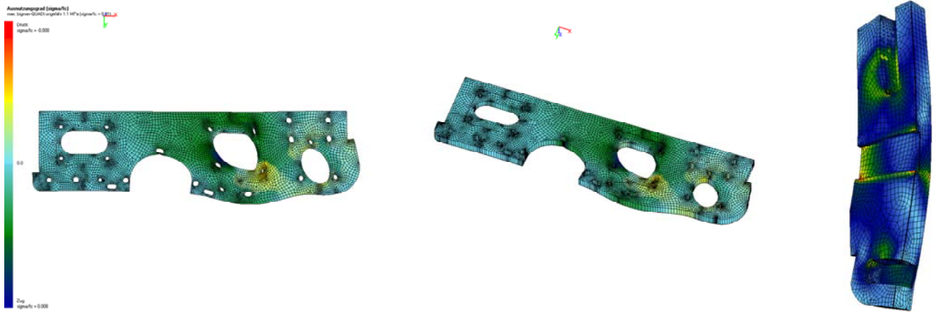
Connection elements – stress analysis.
